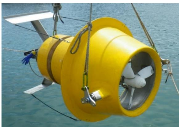
Fig. 14 Floating tidal turbine with diffuser<sup>13)</sup>.
