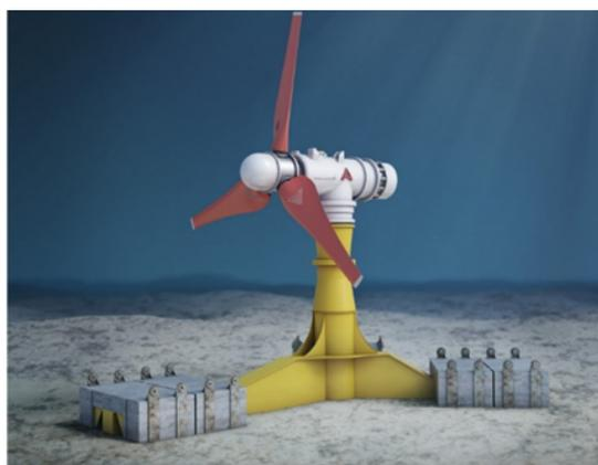
Fig. 5 Tidal turbine for MeyGen project<sup>5)</sup> .
